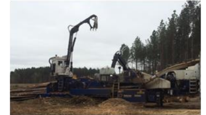
Whole tree disc knife chipper with chain flail
