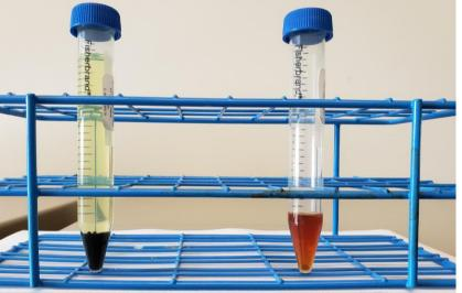
Heavy ends of bio-oil is immiscible in diesel fuel Blend of 18.1% phenyl hexanoate in diesel fuel
