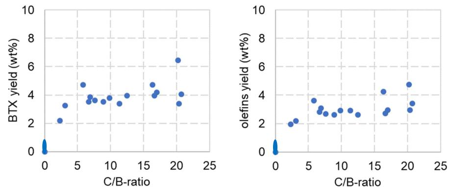
No catalyst → negligible BTX and olefins (ethylene+propylene)
