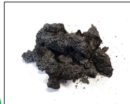
Agglomerated char from acid pretreated biomass
