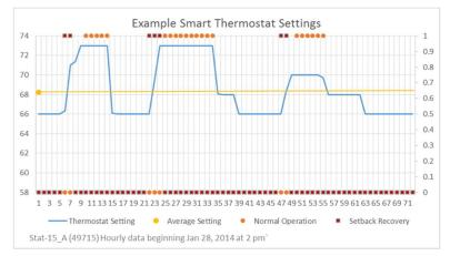
Figure 8: Thermostat Operation With Moderate Frequency and Amplitude
