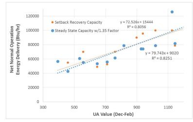
Figure 16: UA Value (Dec-Feb) and Delivered Energy Rate for Steady-State and Setback Recovery
