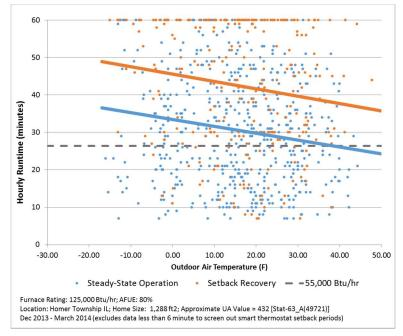
Figure 10: Example Furnace Steady-State and Setback Recovery Operation
