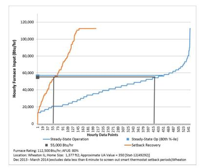
Figure 12: Steady State Operating Mode Hourly Furnace Input Rate Distribution (Wheaton)
