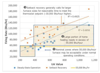
Figure 14: UA Value (Dec-Feb) and Furnace Capacity Requirements
