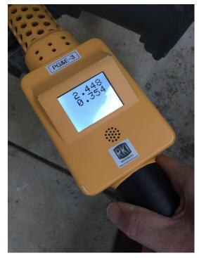
Prototype of the handheld methaneethane detector.
