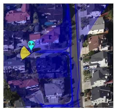
Asset coverage with mobile leak detection, indication of higher methane concentration, coverage gaps
