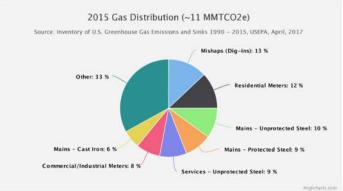
Figure 6. Methane Emissions from Gas Distribution
